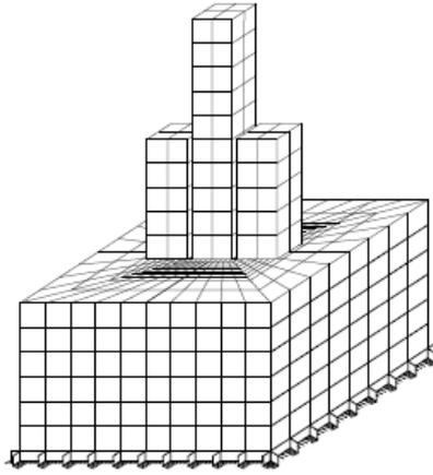
**Fig. 1** Modelling of Structure-soil-structure interaction for a group of three structures in direct method
