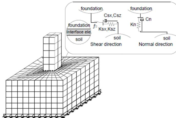
Fig. 2 Interface elements in SSI or SSSI models
